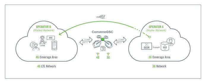
Operators need to contend with the management of traffic for the GPRS Tunneling Protocol (GTP) both the control plane (GTP-C) and the user plane (GTP-U) and versions of GTP between multiple packet core networks. See the GTP types and versions reference diagram at the end of the document.
